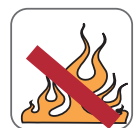
Flame Retardant NF C32-070-2.1(C2) IEC 60332-1/EN 50265-2-1
